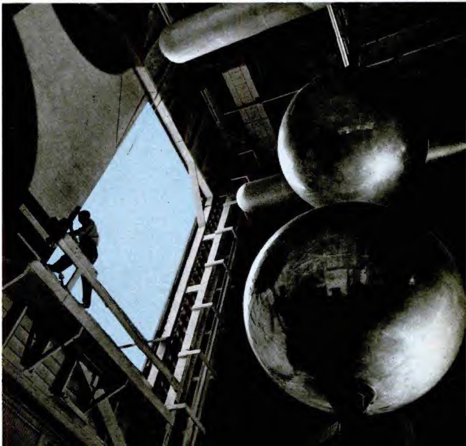
Four million volts of electricity are made to leap across the gap between these two spheres in lightning lab
